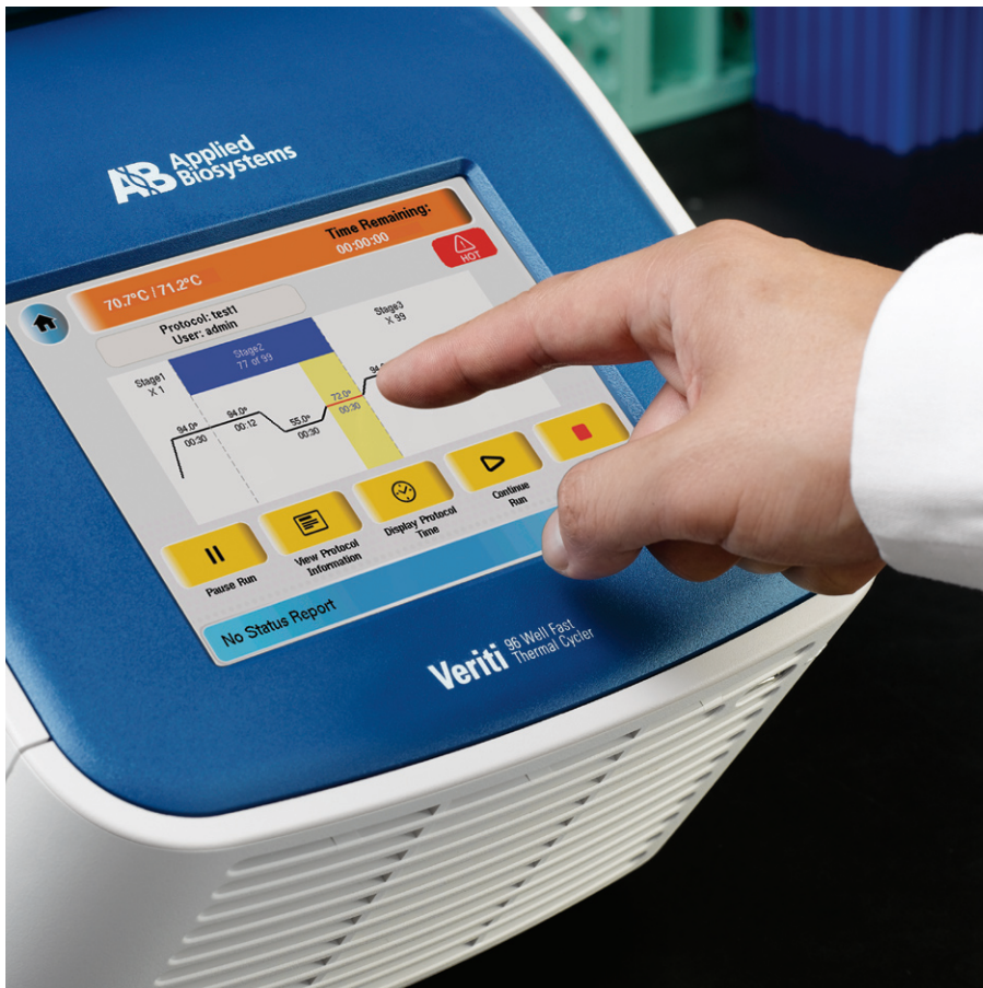
Figure 2. Veriti Thermal Cycler 6.5 inch VGA color touch screen.
