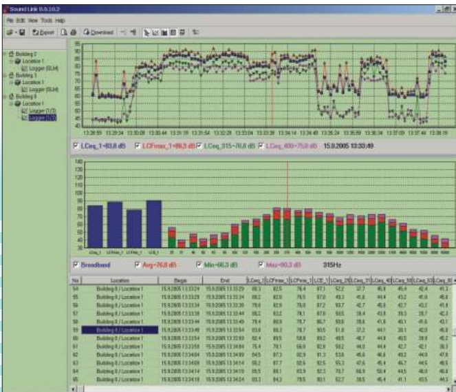
Logged data analysis with SoundLink PRO PC software.
