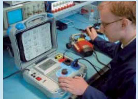
Final test on a portable appliance in a service workshop
