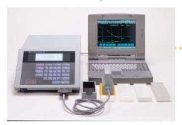
QTM-500 does quick and easy measurement of all kinds and types of sample materials. Stick sensor probe on sample surface of thermal equilibrium, and press START key. The measurement results will appear on display in 60 seconds.
