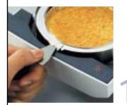
Insert sample holder. The sample drawer opens and closes at a keystroke.
