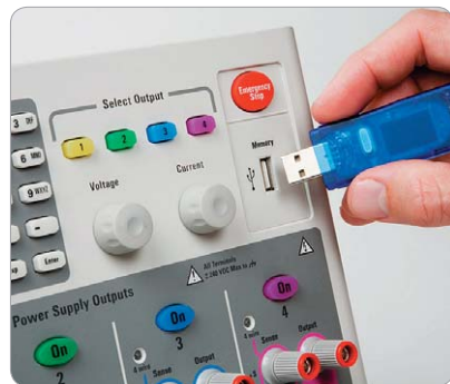
Figure 12. The N6705's front panel USB port
